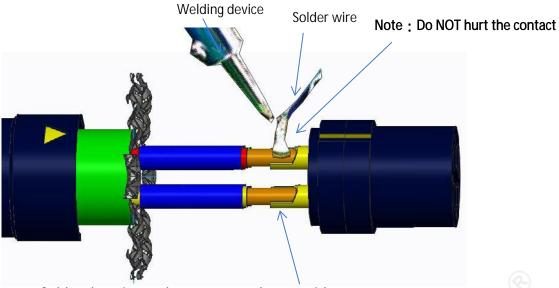
6. Solder the wire to the contact and wrap with HS tube after soldering.
