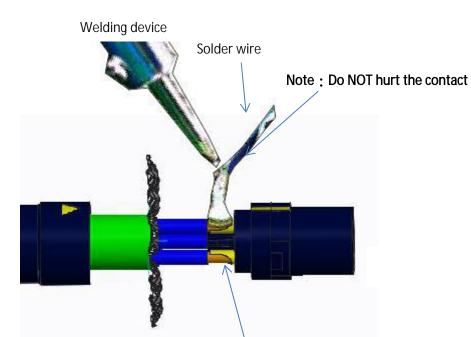
6. Solder the wire to the contact and wrap with HS tube after soldering.
