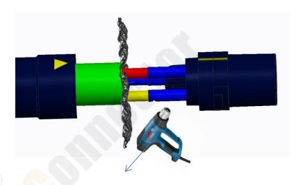
7. Wrap the HS tube tightly by using hot air gun.
